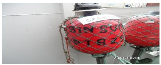
Figure 8. GPS Buoy(M2P)
