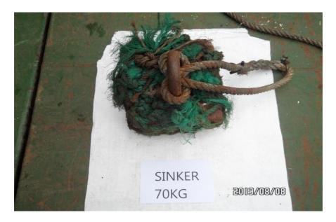
Figure 6. Sinker Weight 70kg
