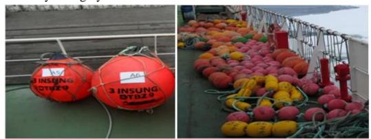
\*Depending on sea-ice conditions (for preventing the loss of fishing gear), either plastic float buoy & eva float buoy or Norway buoy is used.
